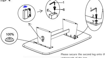
Please secure the second leg onto the underneath of the top. Then fully tighten all the remaining screws
