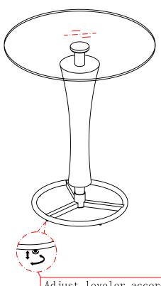
Adjust leveler according to ground level.
