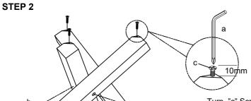
Turn "c" Screw to a point where 10MM is left showing..
