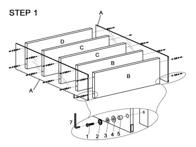
Fasten B, C and D to E, with (1), (2), (3), (4), (5) by (7). Repeat the same step to other 19 screw holes.
