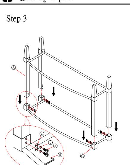
Assemble the frame , and tighten the screw of stretch .
