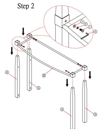
Assemble the stretch , fasten the screws 80% tight.
