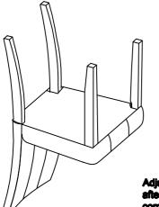
Adjust the product leveled on the ground after upside down, then tighten all screws completely.
