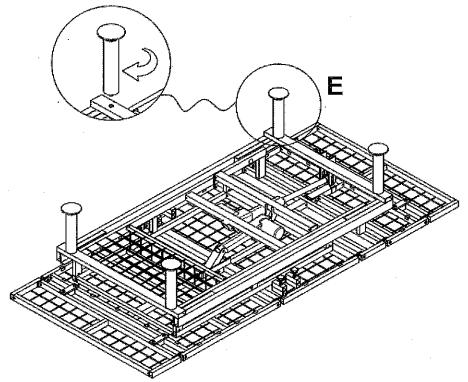
3. Install the 4 legs by turning the legs clockwise until tight. Once all 4 legs are installed, turn the adjustable base over so the legs are resting on the floor.
