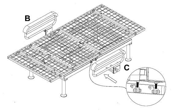
4. Install the hand rail as shown, then turning the plastic screws clockwise until tight.
