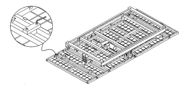
2. Use supplied bolts and wrench, tighten up the frame with the frame connectors as shown.
