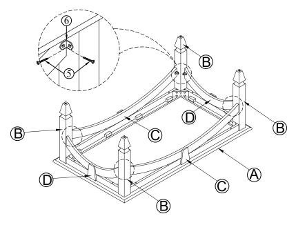
\*PRE-DRILLED HOLE POSITION TO ATTACH METAL CONNECTING PLATE
