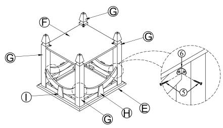
\*PRE-DRILLED HOLE POSITION TO ATTACH METAL CONNECTING PLATE
