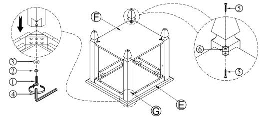
\*PRE-DRILLED HOLE POSITION TO ATTACH METAL CONNECTING PLATE
