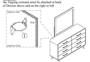
STEP 2: Assembly the tipping Restraint (5).
