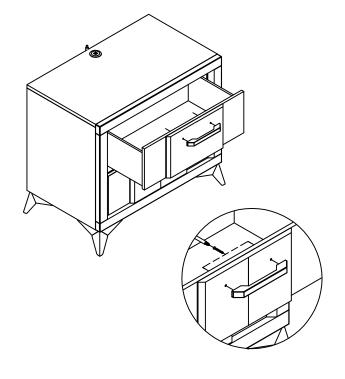
**STEP 3**: Move the Night Stand (A) into final position and use tipping restraint (1) attach to wall
