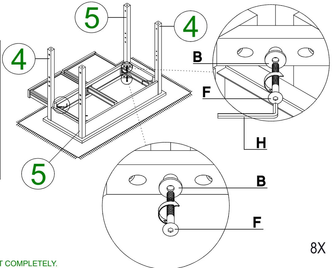
DO NOT TIGHTEN BOLT COMPLETELY.
