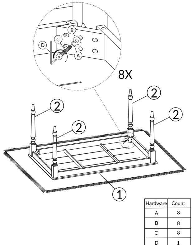
TIGHTEN BOLT COMPLETELY.
