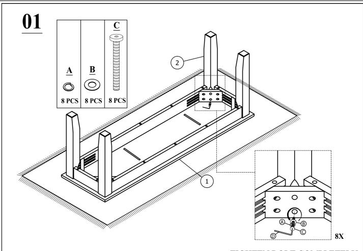
TIGHTEN BOLT COMPLETELY.
