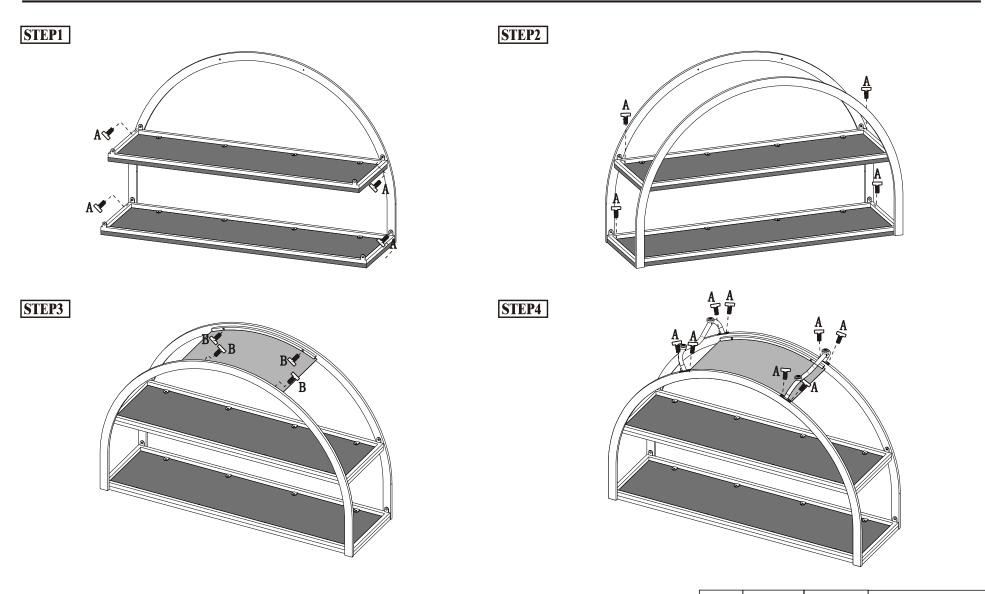
Note:Pls do not tighten all bolts until the products is assembled completely .
