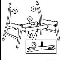
Front Stretcher has a small hole for identification.
