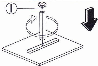
Attach the support leg (P6) to the seat with centre rail (P5). Fix the adjuster (I) to the bottom of the support leg. You will need to use hardware :
