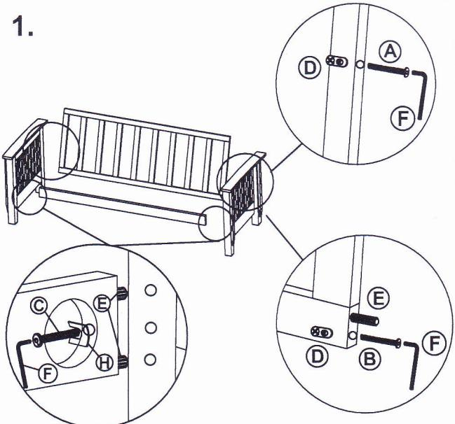
Attach the backrest (P1) and front rail (P2) between the handle (P3). You will need to use hardware:
