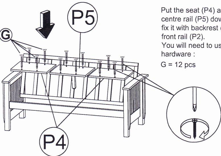
Put the seat (P4) and seat with centre rail (P5) down and fix it with backrest (P1) and front rail (P2). You will need to use hardware :
