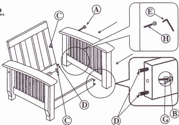
Put the seat panel (P4) down and fix it with backrest (P1) and front rail (P2).
