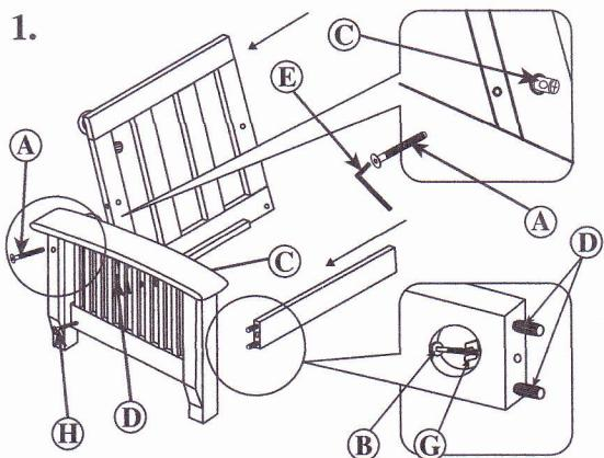
Attach the backrest (P1) and front rail (P2) between the handle (P3).
