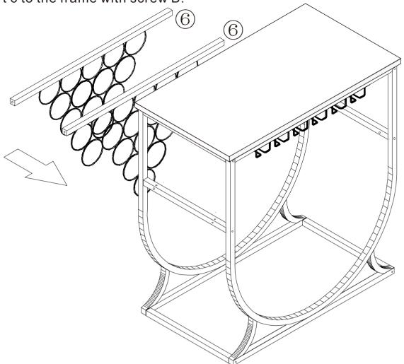
**6** • Fix Part 6 to the frame with screw B.
