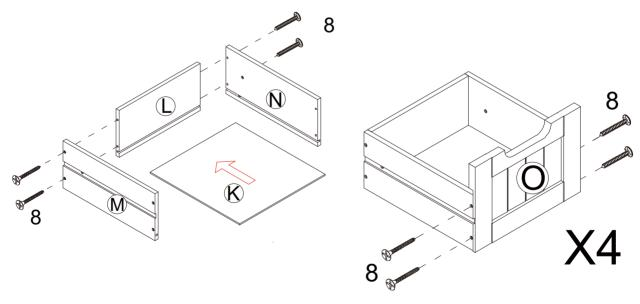
Fix Part N and M to Part L with screw 8, and then put Part K to the groove of Part N and M.
