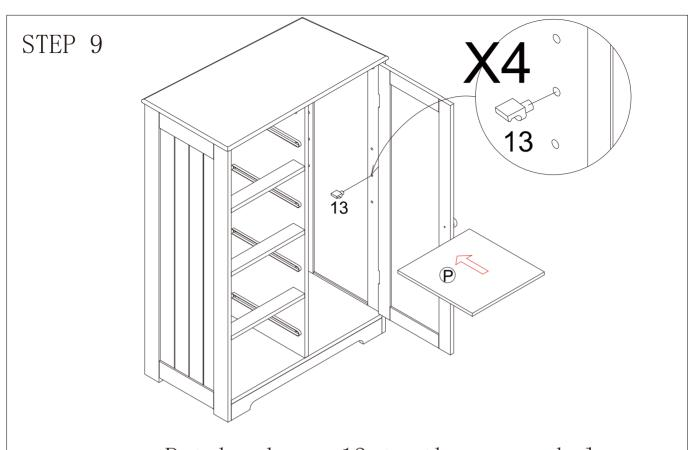
(13)x4pcs Put hardware 13 to the screw hole and then put Part P into the frame.
