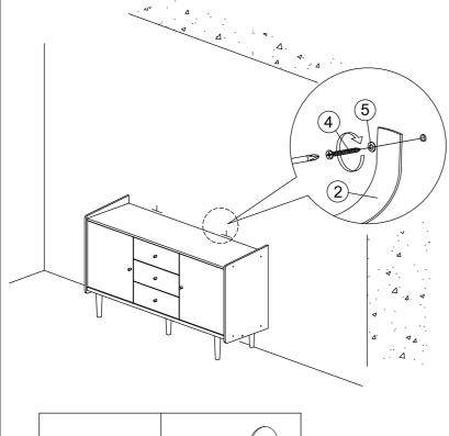
5. Finally, attach safety strap (2) and washer (5) using 4x30mm screw (4) to the wall.
