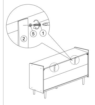
4. Add safety strap (2), washer (5) using 3.5x15mm screw (1) to back of cabinet.
