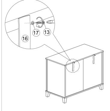
4. Add safety strap (16), washer (17) using 3.5x15mm screw (13) to back of cabinet.
