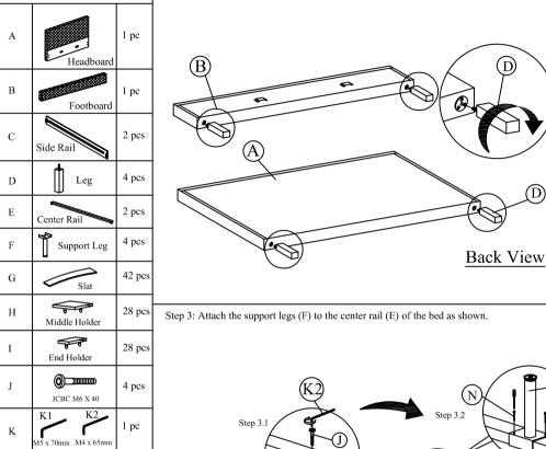
Step 2: Attach side rail (C) to headboard (A) and footboard (B) by pushing the bracket down to fit it.
