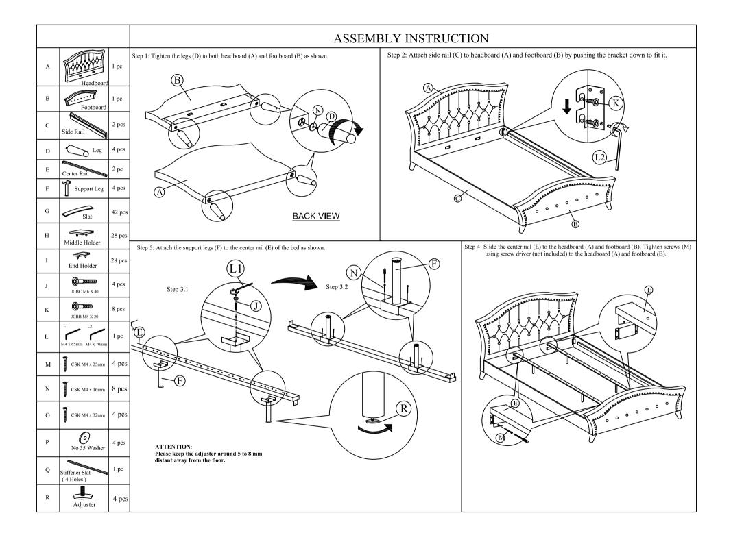
Step 5: Affix the Stiffener Slat (Q) to the side rail support wood and the center rail (E). Tighten all the 4 corner, follow by assembly of the slat holders with LVL slats as shown.
