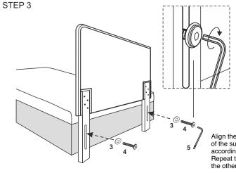
Align the pre-drilled lower holes of the support over the pre-drilled holes on the bed according to your desired headboard height. Repeat the same procedure for the other side.
