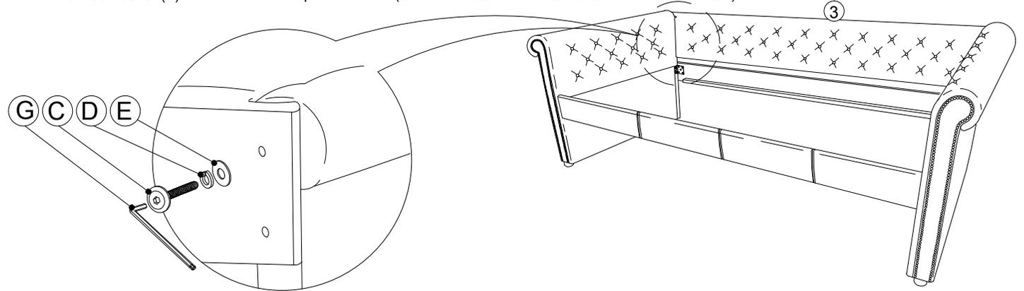
**STEP 4** Tighten all bolts from STEP 2 using the Allen Wrench (F) that has been provided. Now only tighten bolts for STEP 3 using Allen Wrench (G). Attach Slat (6) to Front Rail (4) and Back Rail (5) by unrolling and securing with 4 Wood Screws (A) 2 per each side. Tighten all screws using philips head screwdriver (not included)
