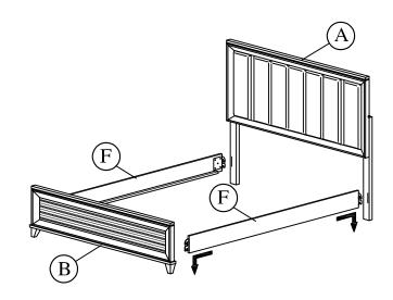
Step 2: Attach the (F) Side Rail to the (A) Headboard & (B) Footboard.
