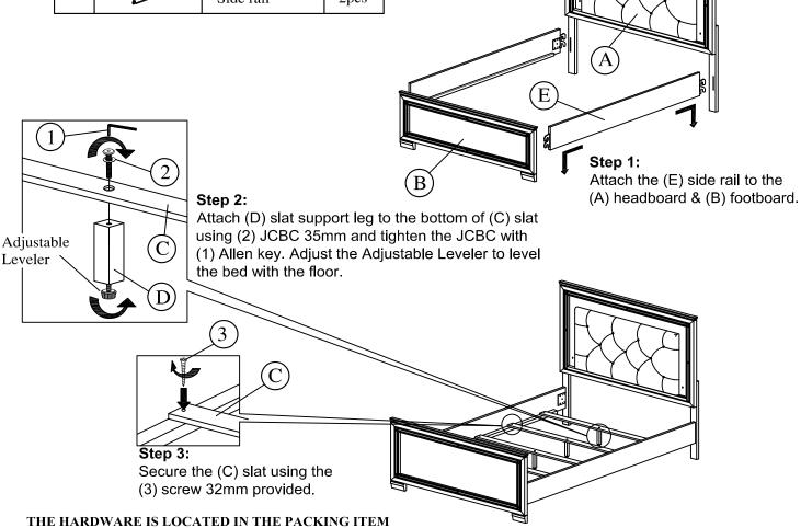
NOTE: MUST TIGHTEN SCREW PERIODICALLY. WITH USE SCREW MAY BECOME LOOSE. CHECK TIGHNESS OF ALL SCREW EVERY 6-8 WEEKS.
