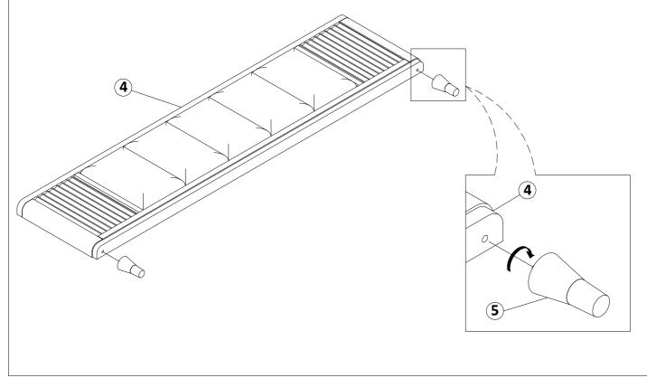
NOTE: MUST TIGHTEN SCREWS PERIODICALLY WITH USE SCREWS WILL BECOME LOOSE.CHECK TIGHTNESS OF ALL SCREWS EVERY 6-8 WEEKS.
