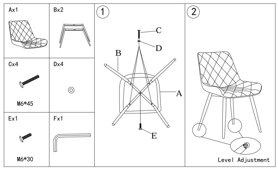
Note: Make sure all screws are fully tightened before using the chair.
