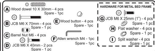
NOTE: WE INCLUDE SPARE HARDWARE IN CASE DAMAGE OCCURS DURING ASSEMBLY.
