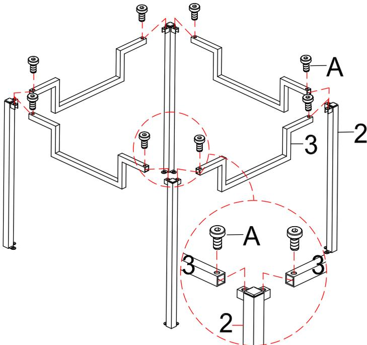
Attach bottom stretchers (3) to legs (2) using bolts (A) as shown.
