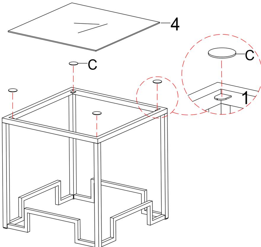
Attach glass pads to top frame (1), then put glass top (4) to top frame (1) as shown.
