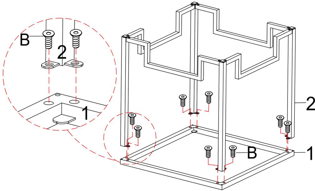
Attach the assembled unit to top frame (1) using bolts (B) as shown.
