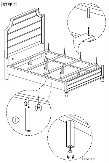
**WARNING**: Do not tighten up the bolt in one side for this step, until all bolt and part is properly assembled.
