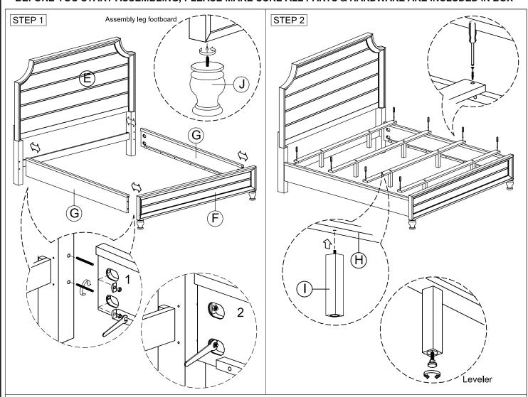
**WARNING**: Do not tighten up the bolt in one side for this step, until all bolt and part is properly assembled.
