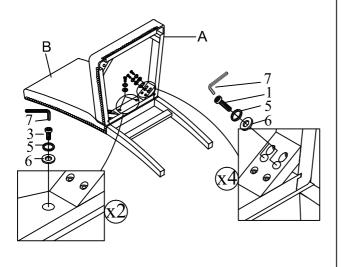
STEP 2 :Insert Front Legs into Seat Frame One Side At a Time
